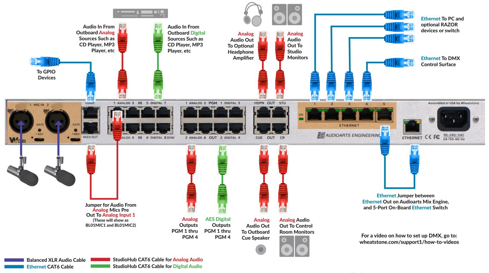
Think of the back of the Audioarts Mix Engine as a rack that has a TWO CHANNEL MIC PRE, an I/O SECTION, and a 5-PORT ETHERNET SWITCH mounted in it. To use them, you have to physically patch the outputs of the MIC INPUTS into your choice of ANALOG INPUTS 1-4 (Input 1 is pre-configured for this). Likewise, to use the Audioarts Mix Engine with the 5-port switch, you need to physically jumper the ETHERNET OUT to an available port on the onboard 5-port ETHERNET switch.
