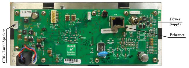
To make power and Ethernet connections for the Talent Station desk panel plug the power adapter and Ethernet cable into the power connector and the RJ-45 located on the rear of the unit.
