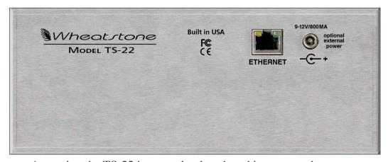
Assuming the TS-22 is properly placed, and its power adapter connected to the unit, you may now energize the unit by plugging it into the AC mains. The TS-22's switches will assume factory default settings.
