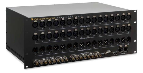
The optional 4RU StageBox One is for extending console I/O, providing 32 mic/line inputs, 16 analog line outputs, and 8 AES3 inputs and 8 AES3 outputs as well as 12 logic ports and dual Ethernet ports. StageBox One works with all WheatNet-IP audio networked consoles.
