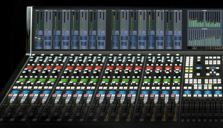
With all I/O managed through a separate rack unit, Wheatstone control surfaces have no limitations with fixed connection points on the console chassis itself. Any channel can connect to any audio source, using any preferred audio format at any time, whether it's HD/SDI, AES, MADI, AoIP, Analog or TDM.
