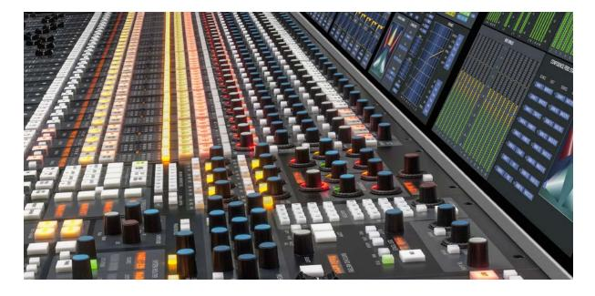
down-mixing between stereo and 5.1 sources, plus a full complement of stereo and 5.1 surround panning with EQ and dynamics processing available for each input, each subgroup and each program bus. For overall control, this control surface uses motorized faders, each of which can be mono, stereo, or full 5.1. Each fader also has a "spill" function, which allows its individual channels to spill out onto separate faders (two for stereo or six for 5.1 sources).
