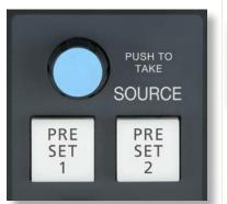
With Preset 1 and Preset 2 source selectors provided on each fader, if the primary feed goes silent, an operator need simply press the second source to recover audio. Because the system supports such a vast number of inputs, there's room to provide these redundancies without the need for patching or external switching.
