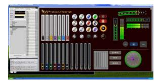
ScreenBuilder™GSX comes stocked with widget graphic elements: meters, faders, knobs, buttons, tallies, etc., all ready to drag, drop, and configure. You can also add your own graphics, and assign functions to them using our script wizard. We've seen studio mic plots, simple on/off talent panels, even maps of entire countries showing all transmitter locations - it's pretty much wide open. If you can conceive it, you can achieve it.
