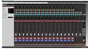
Here's how it works: the display shows you the layout of your physical console - just double click on the surface feature you want to customize (switch, knob, fader, OLED display) and using the drop-down menu, select the function you'd like to assign to it. If you require more complex programming, you can even script things to achieve the exact level of control you need. Many GSX GUI functions can be customized as well.
