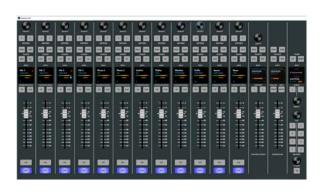
Working in conjunction with the GSX hardware surface, Remote GSX provides complementary production functions for separate operators using an GSX board in the same location or in another location over an IP connection. Real-time fader tracking and live synchronization of buttons and controls between the virtual surface and the physical GSX board offer an independent, yet shared user experience for multiple operators – or as a tool for engineers to remote in to correct operator setup issues.
