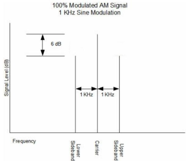
When the modulating signal causes the carrier to be 100% modulated the amplitude of the carrier is reduced to zero during the negative excursions of the audio waveform, and during positive peaks it reaches twice the carrier-only value. The resulting modulated RF carrier looks like this.
