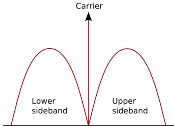
At 100% modulation the signal is made up of the RF carrier at the station's assigned operating frequency and a pair of sidebands corresponding to the audio modulation; each sideband contains 25% of the power of the carrier. That is, the sidebands are 6dB (in voltage amplitude) below that of the carrier when the carrier is modulated to 100%.
