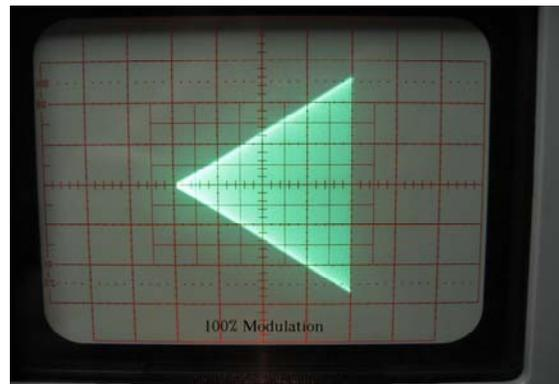
The near-perfect linearity shown in the above photos demonstrates the kind of audio performance required to provide high modulation levels and high signal quality simultaneously.
