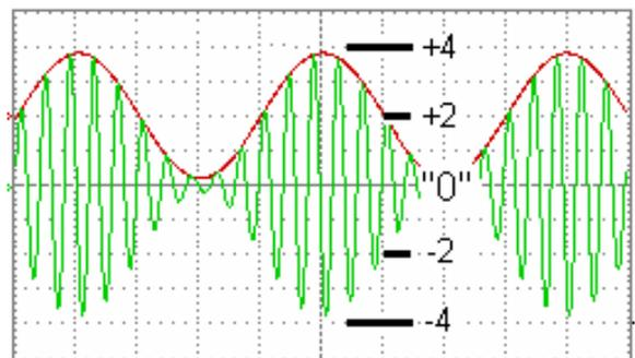
We have just seen that at 100% modulation the peak modulated RF carrier voltage (**E**) is *twice* the carrier-only value (hang in there – this is important!). Since the value of load resistance is fixed (let's use 50 ohms in this example) the RF *current* (**I**) into that load resistance must also be *twice* the carrier-only value.
