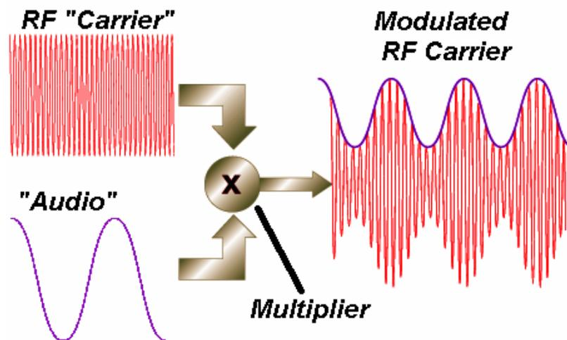
The output of this scheme is the modulated RF envelope we spoke of earlier which can then be demodulated by an AM receiver tuned to the RF carrier's frequency.
