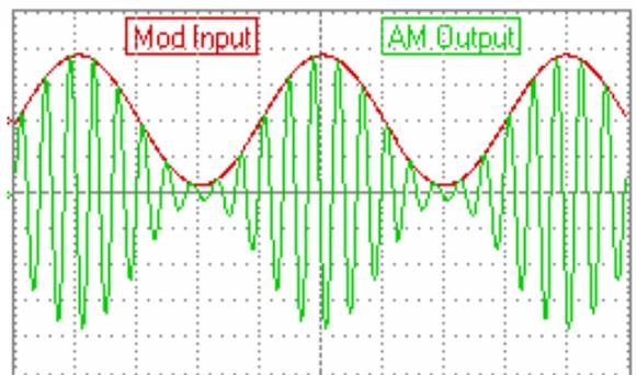
Therefore at 100% modulation the RF carrier will be swinging between zero and twice the carrier value as shown. 100% modulation is shown here as the waveform reaching +/-4 units in amplitude where the un-modulated carrier by itself would just be +/- 2 units.
