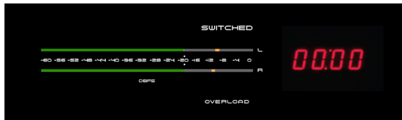
Figure 4-6 Meter Bridge, Switched Meter and Timer
