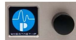
Figure 2-11 Razor front panel OLED and Encoder
