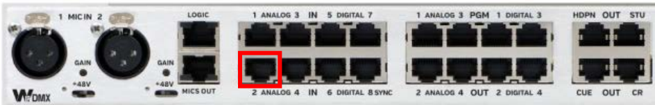
Figure 2-8 Mix Engine, rear panel partial, showing Audio and Logic Jacks
