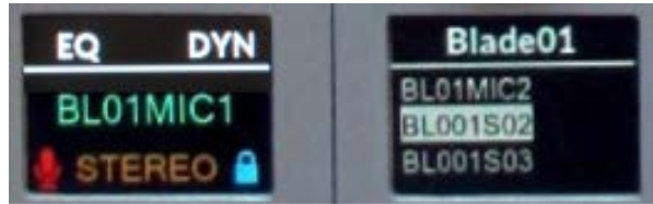
Figure 4-3 Channel Displays: Left = Normal (Source Name & Status) Right = Selecting a New Source (Alternate Source Name List)
