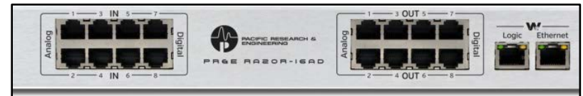
Figure 1-7 Razor 16AD Interface, Rear Panel RJ45 Connectors
