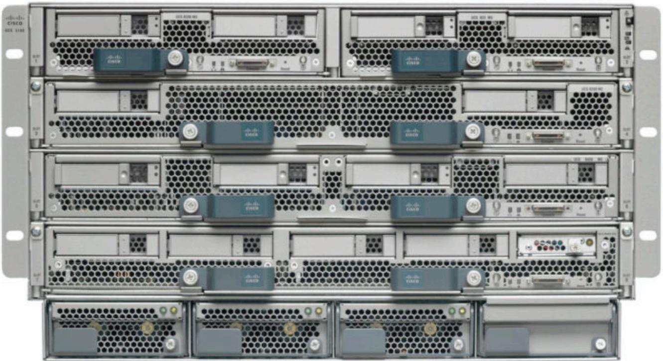
*Example of a Cisco server blade stack, which can be managed by a hypervisor and output to a fabric interconnect that hooks to an AoIP switch.*
