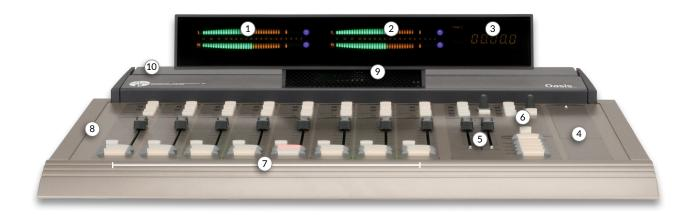
Part of the PR&E portfolio, Oasis™ is a high-value standalone audio console for on-air and radio production applications. Simply connect microphones, source equipment and audio monitors — even a PC automation channel (no sound card required) — directly into the Oasis console and be on the air.
