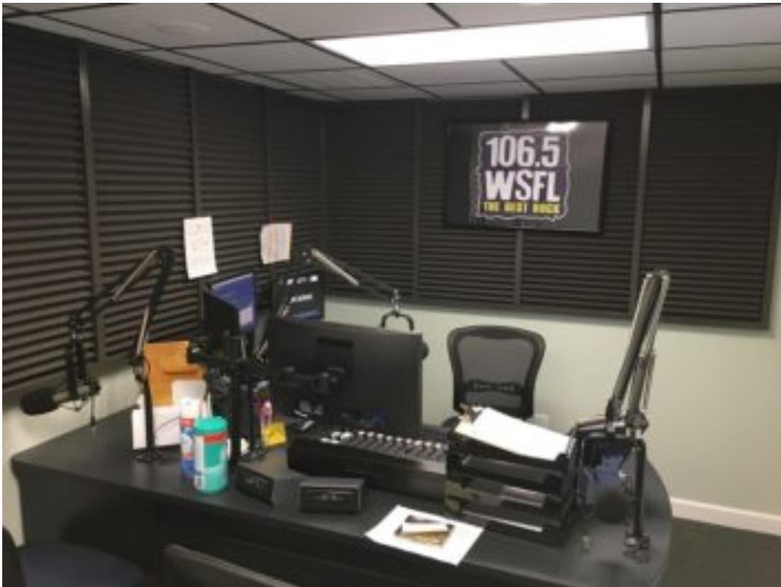
We dropped into the furniture Wheatstone's IP-12 control surface with mixing engine, M4IP-USB mic processor
