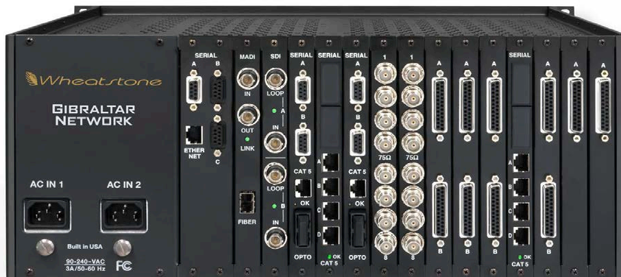
On the Gibraltar Network and Gibraltar IP Mix Engine cages, power supplies are internal and can be single or dual modules. The back provides access to the cards' connections.
