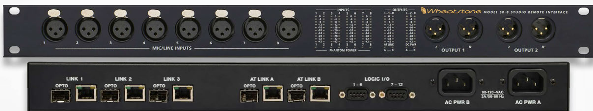
The SR-8 provides eight XLR inputs and four XLR outputs in a stage-box configuration. It interfaces to the Gibraltar Network via CAT-6 cables and comes with dual internal power supplies for redundancy.
