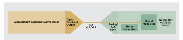
Wheatstone® baseband 192 digitizes the entire multiplex spectrum including RDS and SCAs up to 80kHz, providing a higher performance interface than using the classic analog composite method between processing and transmitter. A single AES/EBU cable between the processor and a current solid-state FM transmitter carries the digital baseband signal, bypassing the need for multiplexing in the exciter and eliminating the resulting signal overshoot with its associated loudness tradeoff.
