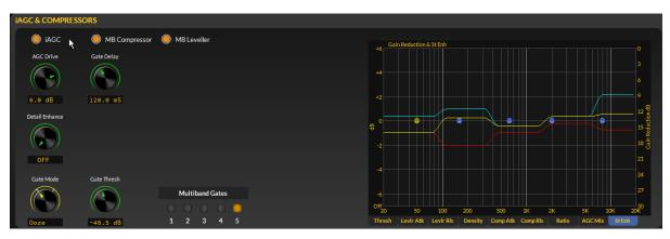
Our adaptive iAGC – or intelligent AGC – allows unobtrusive transitions between hyper-compressed recordings and those with more dynamic range. Effectively manages the behavior of the multiband AGC as program content density changes, something a typical broadband AGC simply cannot do. By coupling the iAGC and multiband AGC, we are able to produce a consistent, spectrally-balanced sound regardless of density variations in incoming source material.
